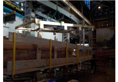
Above left and middle shows the guys rebuilding the 'top hat' and far right it is being craned up into position. Below left the 'box' is complete and is firmly holding the hull in position ready for the rolling process which can be seen in the next two
