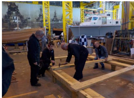
Above left and middle shows the guys rebuilding the 'top hat' and far right it is being craned up into position. Below left the 'box' is complete and is firmly holding the hull in position ready for the rolling process which can be seen in the next two
